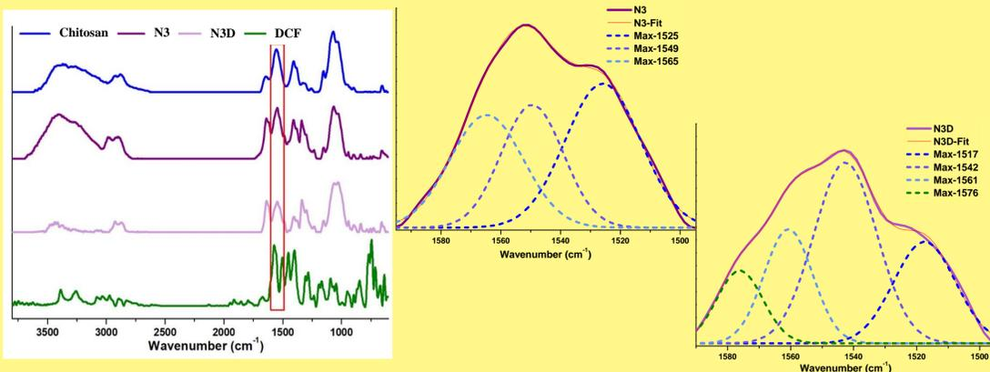
Figure 1. Comparative FTIR spectra and deconvolution of the 1620-1480 cm<sup>-1</sup> spectral domain
